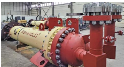
Ultra high pressure heater for a large petrochemical production
