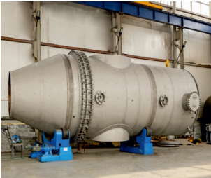
Gas-gas heat exchanger GreenTube Increasing the heat transfer efficiency by 30% while maintaining the specified dimensions
