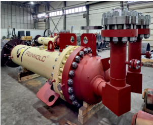
Ultra-high-pressure heater GreenTube Design pressure - 18 MPa
